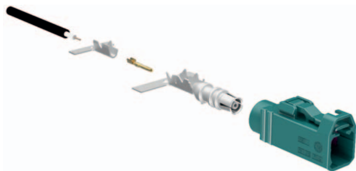
Cable SF support sleeve SF center contact SF connector body Plastic housing
